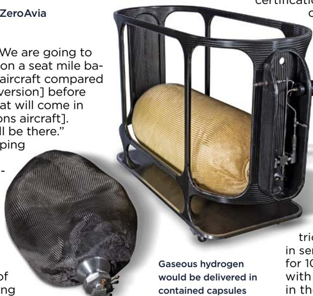
Gaseous hydrogen would be delivered in contained capsules
