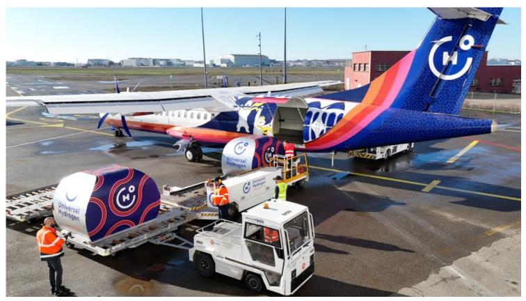
Loading a Universal Hydrogen module onto a plane. Source: Universal Hydrogen Co.
